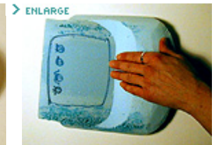
An early prototype of a shared family calendar. The interaction of pushing the product open became a theme which led to a less traditional, more aesthetic product form.
